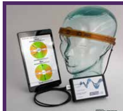
Fig. 3 (bottom). B2v2®, self-use device for closed-loop self-optimization of brain activity (photo courtesy of Brain State Technologies, Scottsdale, Arizona).
